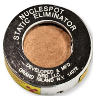
Fig. 10. Po-Be neutron check source: a Nuclespot P2042-1000 static eliminator is paired with a circular thin beryllium window covered with a brown cardboard plug.
