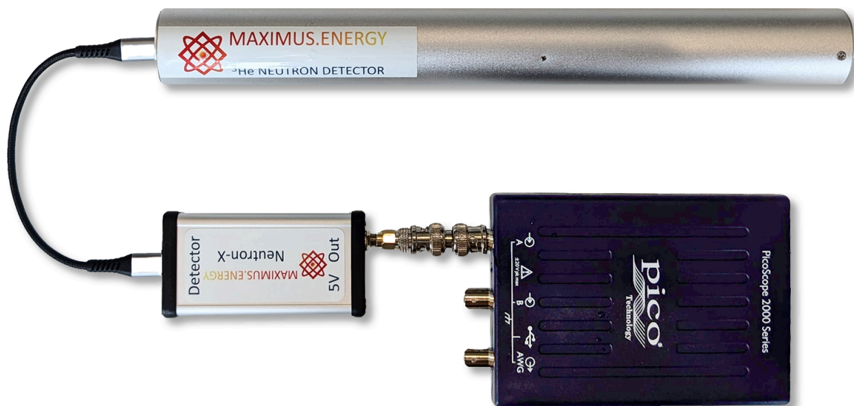
Fig. 5. Low-cost neutron detection architecture.
