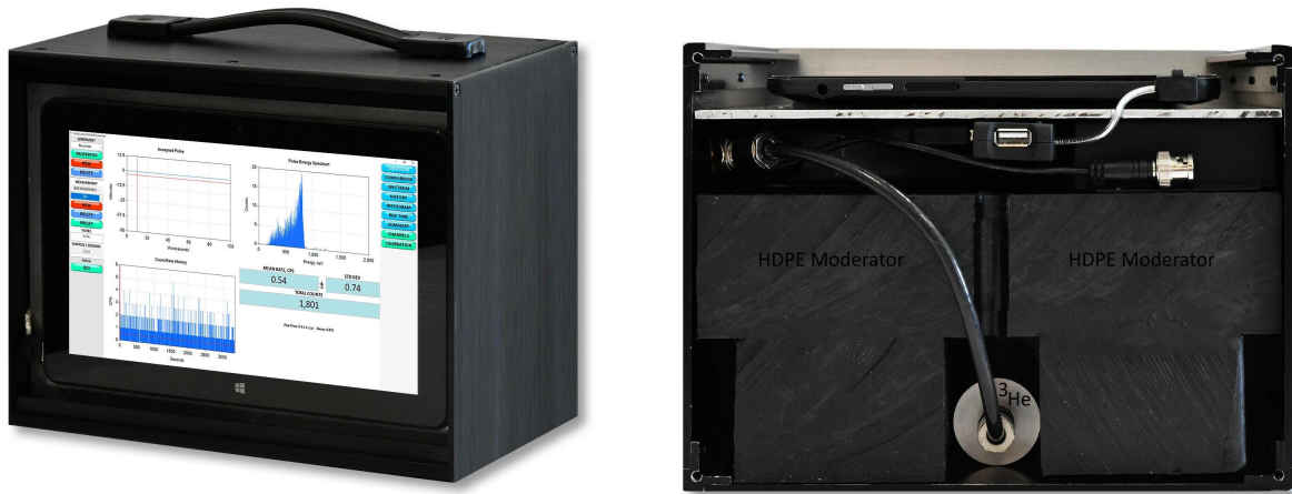
Fig. 10. A Neutron-Pro system featuring the entire detector hardware packaged within a solid aluminum enclosure for maximum EM interference protection.
