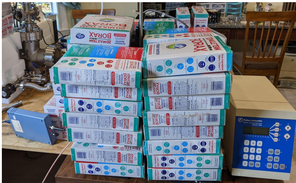
Fig. 12. Borax castle around the neutron detector and the experimental setup.
