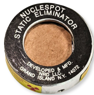
Fig. 8. Po-Be neutron check source: a NucleSpot P2042-1000 static eliminator is paired with a circular thin beryllium window covered with a brown cardboard plug.
