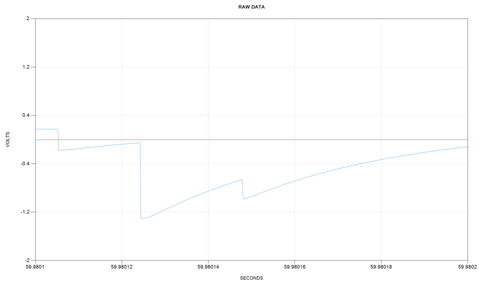
Fig. 2. Long negative step-like pulses from a Canberra resistive feedback charge sensitive preamplifier connected to an HPGe detector.
