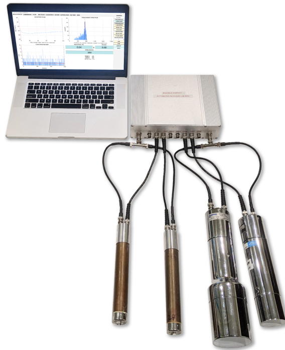
Fig. 1. The Automated Nuclear Lab system: sample configuration with two 3 He proportional neutron counters and two NaI(Tl) gamma scintillation detectors.
