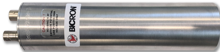
Fig. 5. A gamma detector with an SHV bias-in and a BNC signal-out connectors.
