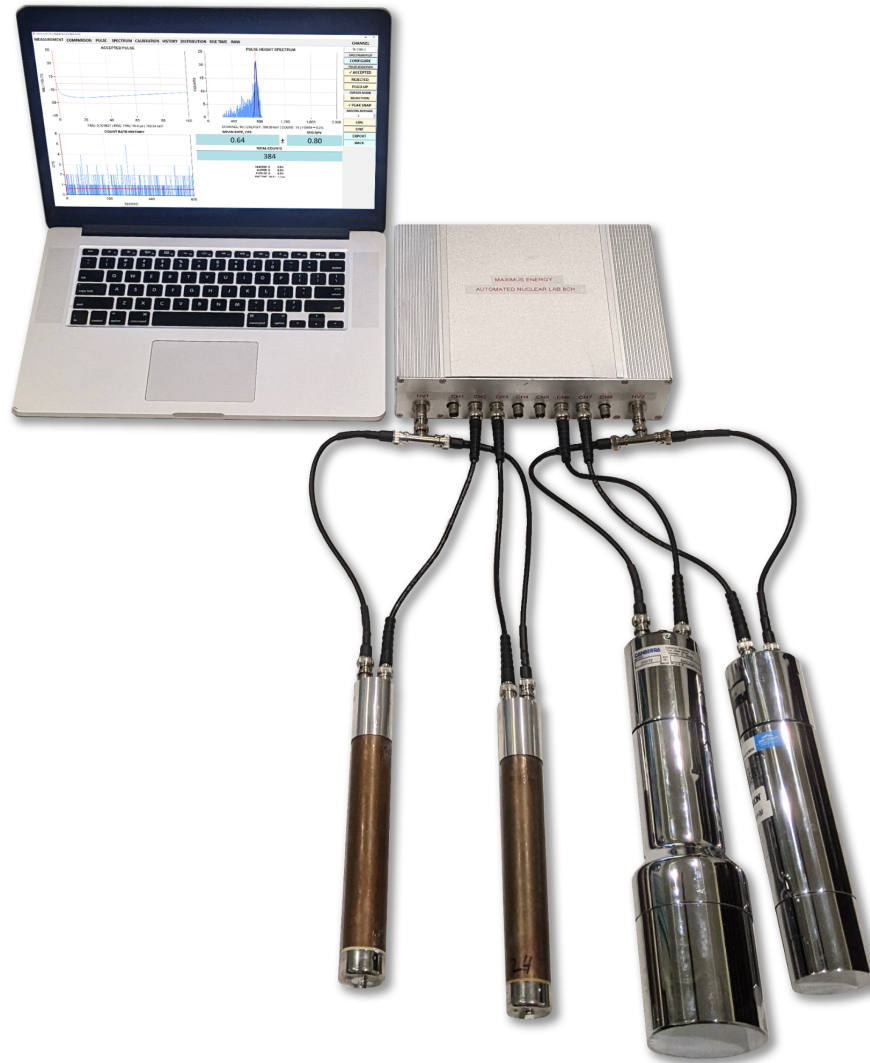
Fig. 4. A sample complete ANL configuration with two ^3\text{He} proportional neutron counters and two NaI(Tl) gamma scintillation detectors.
