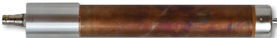
Fig. 6. A neutron proportional counter with a single signal / bias SHV connector.
