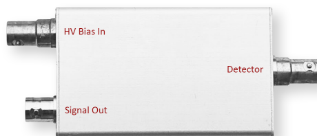
Fig. 9. A bias / signal splitter.
