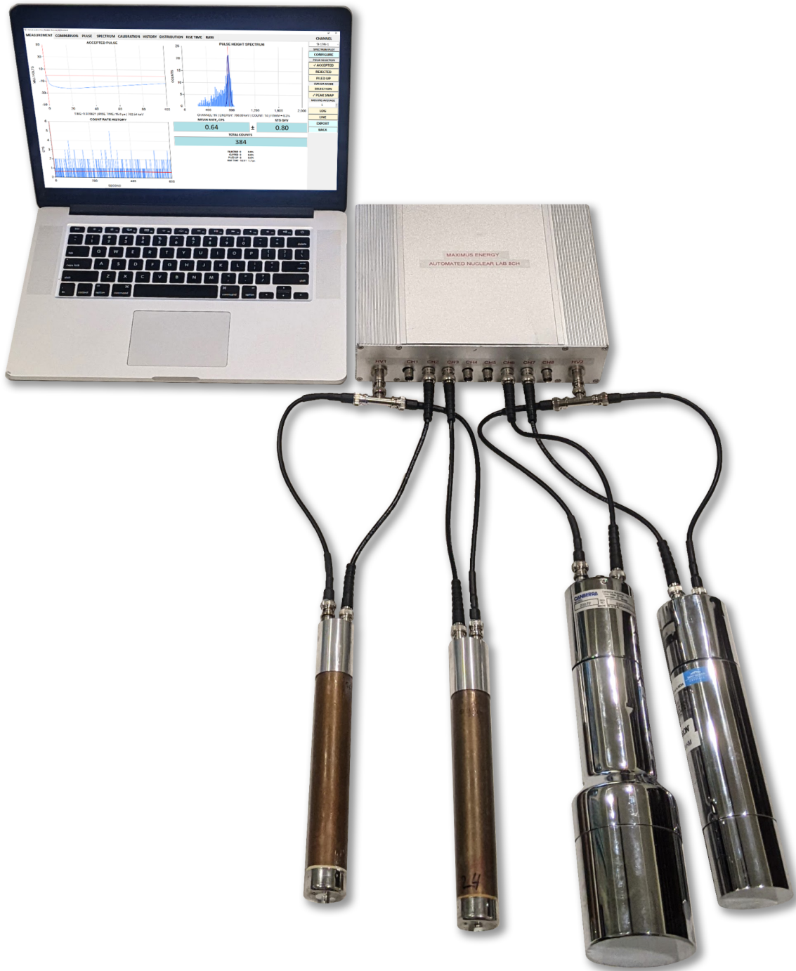
Fig. 2. A sample ANL configuration with two ^3\text{He} proportional neutron counters and two NaI(Tl) gamma scintillation detectors.
