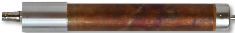
Fig. 8. A neutron proportional counter with a single signal / bias SHV connector.
