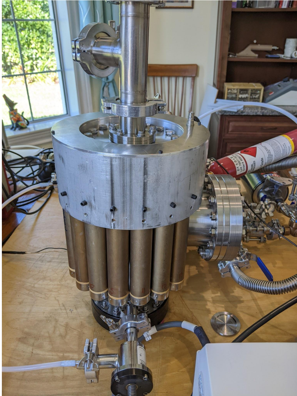
Fig. 4. Closeup of the reactor lined with SI-19N neutron detectors.
