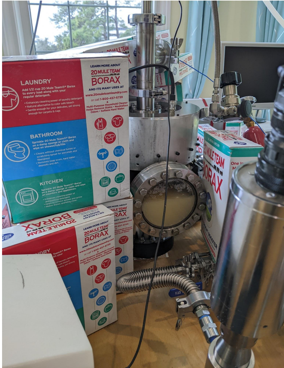
Fig. 7. The reactor shielded with the boxes of Borax.
