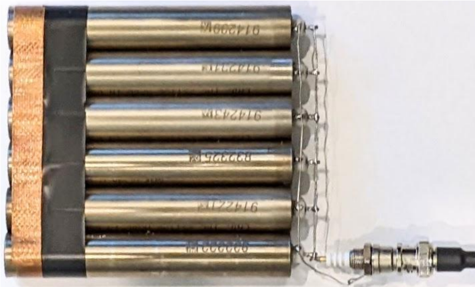
Fig. 5. The bank of six LND 251106 neutron detectors.
